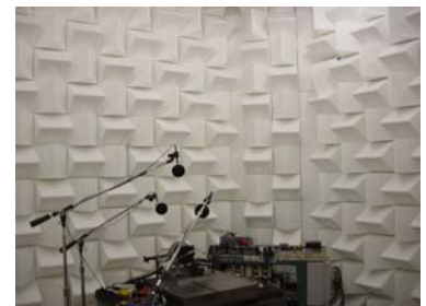
Anechoic Room Interior
