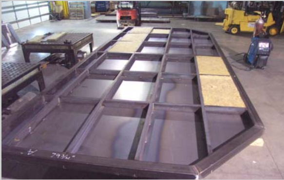
Custom Base Section Being Fabricated
